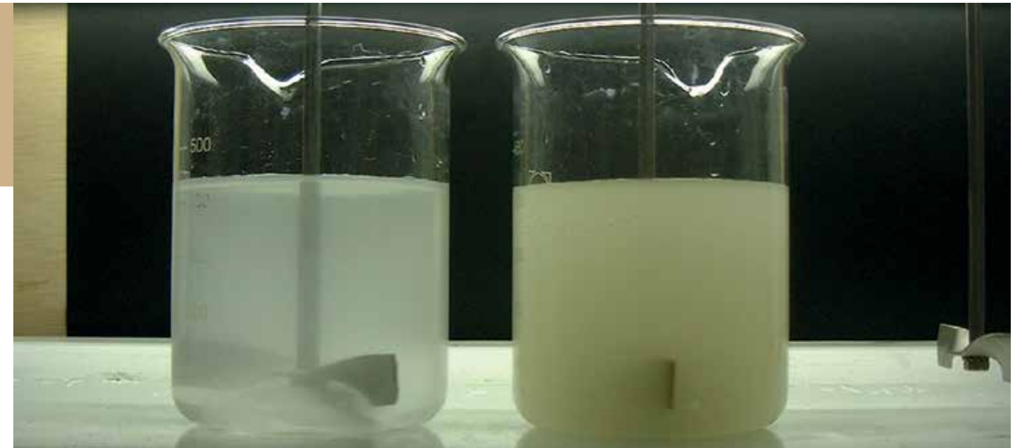
SoluPotasse® (left) dissolves rapidly and completely to give a clear solution, unlike poor quality water-soluble SOP products (right)
