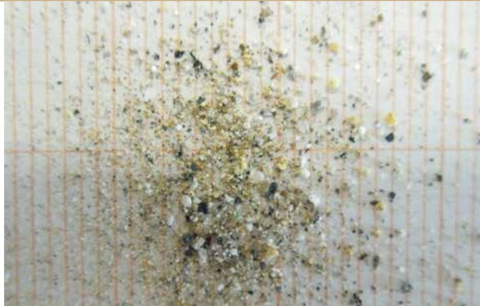
Insoluble material will block the drippers and filters
